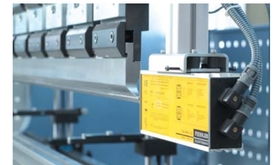
Ce Laser Safety System
